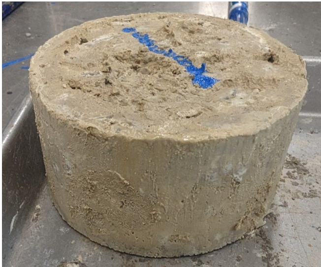
0.75% polymer after molding and before curing
