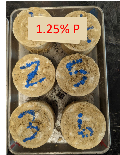
Cured specimens after curing and before conditioning
